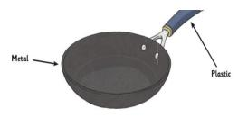
Materials: **Metal-** to **conduct** heat from the hob and allow food in the pan to heat up and cook **Plastic -** to insulate against the heat, so that you can hold the pan without getting burnt.
